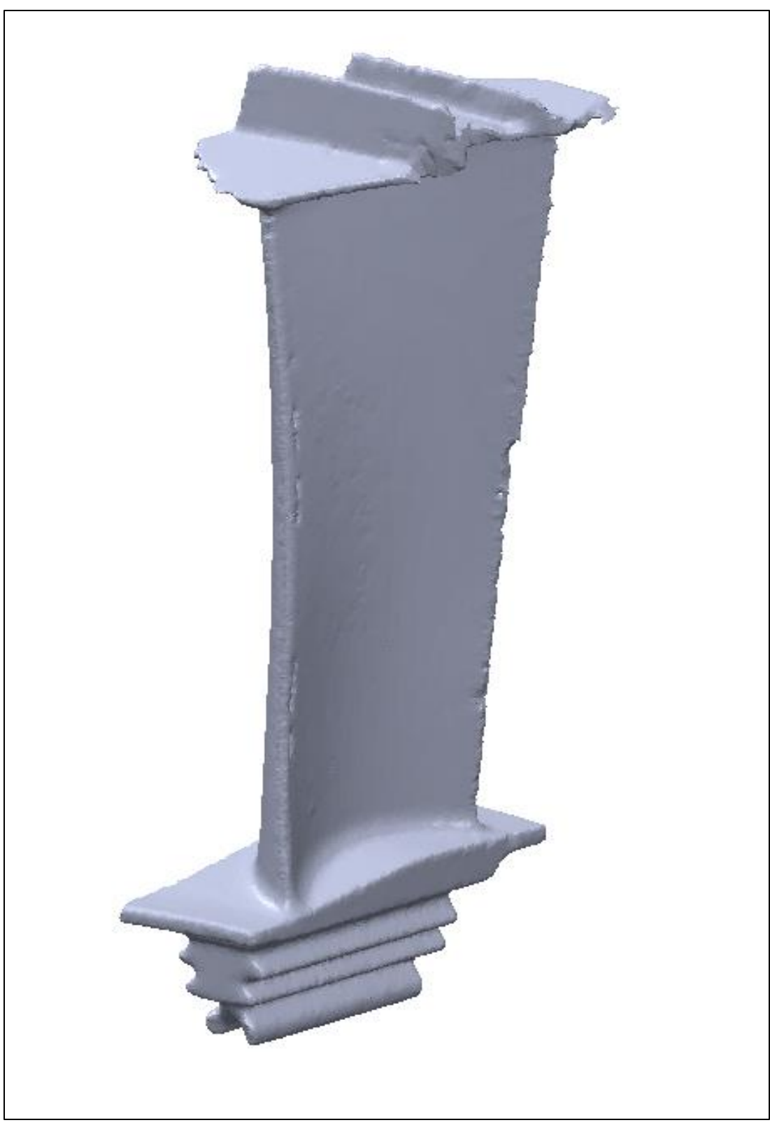
Figure 2 :3D scan of a turbine compressor blade
