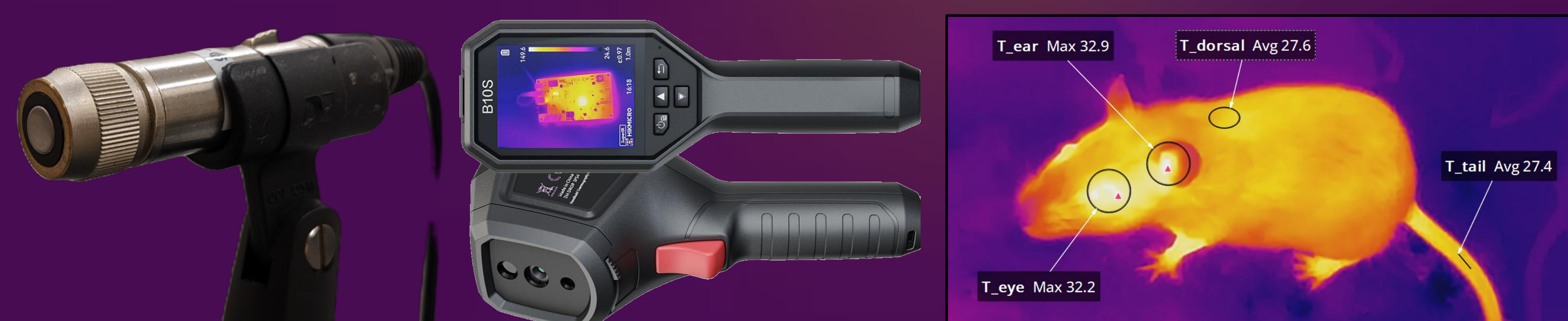
Figure 3. L-R: Avisoft Bioacoustics 40 kHz signal generator, HIKMICRO B10S infrared thermography camera, representative image of rat temperature measurements
